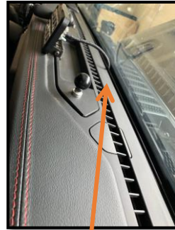
Bring cable up and leave enough cable to attach to the controller and then tilt windshield back up
