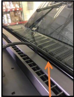
Tilt the windshield forward just enough to pass the cable down into the bottom of the windshield threshold
