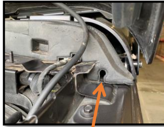
Pass cable through here
