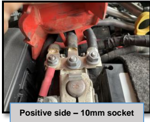
Positive side – 10mm socket
