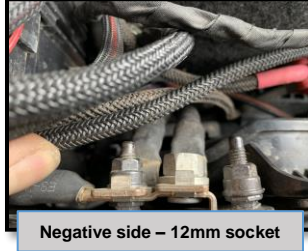
Negative side – 12mm socket
